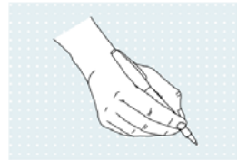
Pencils and pens small diameter, smooth surface > precise gripping
